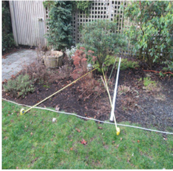
LAYOUT WITH TAPE BASELINE, 10 FOOT VERTICAL BASE LINE AND TRIANGULATING TAPES
